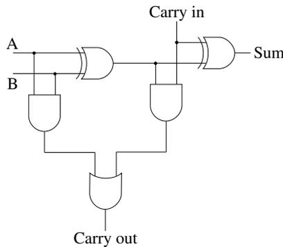
It involves some internal conductors that are not connected to the circuit's external connectors. In the Prolog version, these conductors are replaced by variables that recur in the subgoals of the body but do not occur in the head, here X, Y, and Z.
