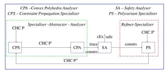
Figure 3: CHC verification toolchain.
