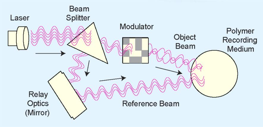
Data is retrieved by passing the reference beam through the hologram, thereby reproducing the original coded object beam.
