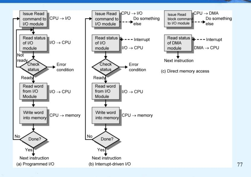
This is an idealized I/O subsystem that uses interrupts.
