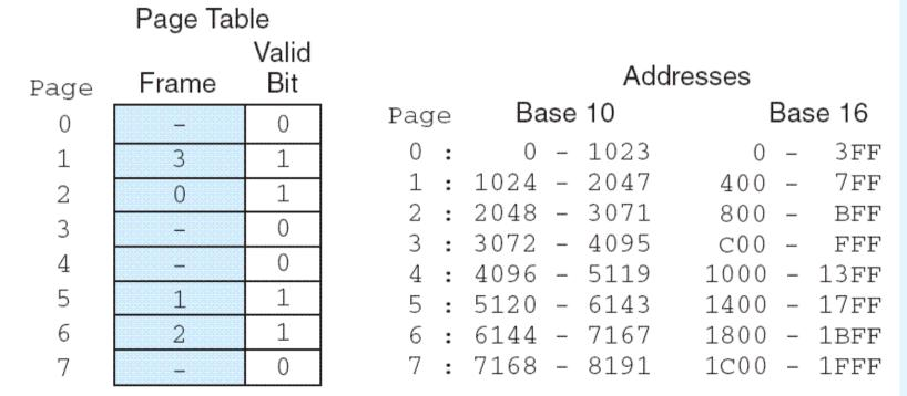
• The address  $1010101010011_2$  is converted to physical address  $010101010011_2 = 1663_{16}$  because the page field 101 is replaced by frame number 01
