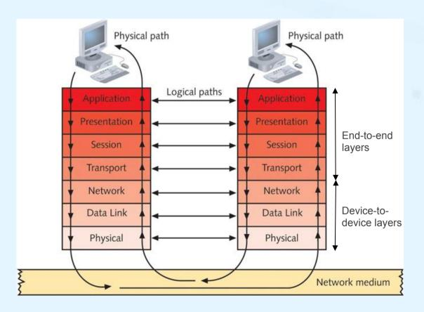
These layers only exist in the host processors at the ends of the connection.
