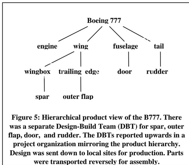
Geographical distribution of component manufacturing was the rule in the 777 project. The components discussed in this paper, shown above in Figure 5, were produced at distant sites. The doors were produced in Japan (by Mitsubishi) and one engine alternative in England (by Rolls Royce). Spars were produced by a subcontractor located 30 miles away from
